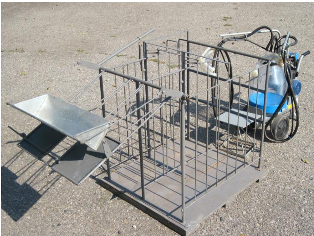
1. "Milk Line" Fig. 1. Two places installation for milking sheep with "Milk Line" components
